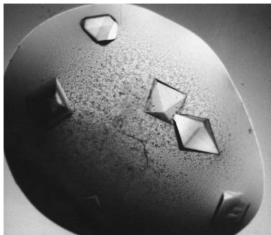
Figure 1 Photograph of tetragonal form I crystals of acetone cyanohydrin lyase from M. esculenta (MeHNL) obtained with PEG 8000 and MPD. The largest dimension of the crystals shown is 1.0 mm.
